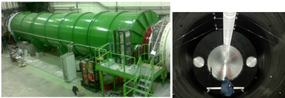
Figure 2.9: The RICH vessel installed in the NA62 cavern (left). The beam pipe seen from the inside of the RICH vessel where the entrance window and the PMT flanges are well visible (right) [47].
