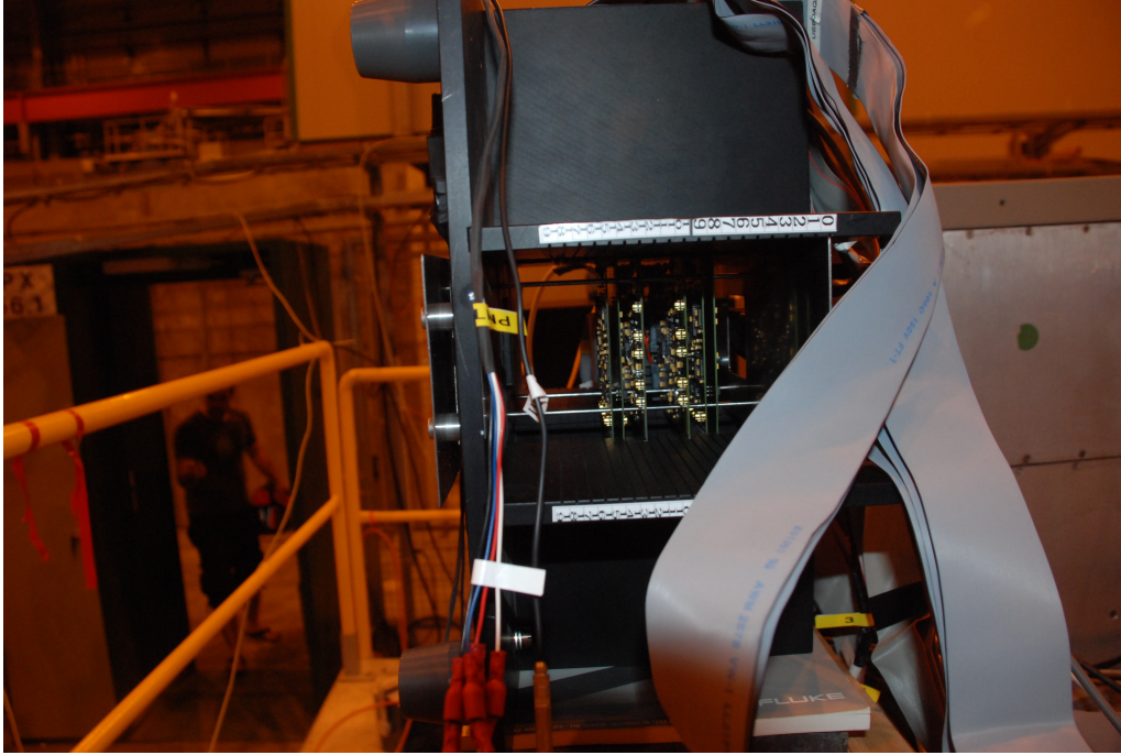
Figure 3.4: Photograph of the TPAC stack setup in tracking mode during the CERN beam test showing six sensors in the TPAC stack with the guide rods visible through the sensors, and the ribbon cables used for readout. The beam is incident from the left of the photograph.
