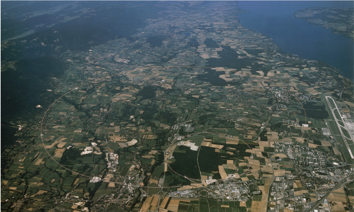
Figure 3.1: Aerial photograph of the countryside next to lake Geneva. The path of these underground CERN accelerator rings are superimposed, in order of increasing size the Proton Synchrotron, Super Proton Synchrotron and Large Hadron Collider. ©CERN.
