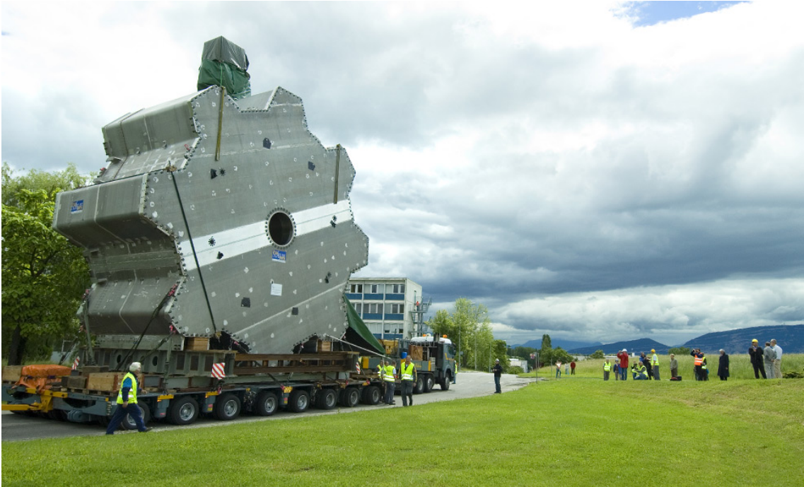
Figure 4.2: The ATLAS A side endcap toroid magnet en route to installation. ©CERN.
