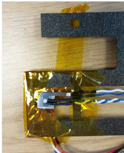
Figure 3.20: Photograph of the mini/finger set up. Finger uninsulated. Two white Pt-1000s can be seen in the centre of the mini-sensor and on the end of the finger.
