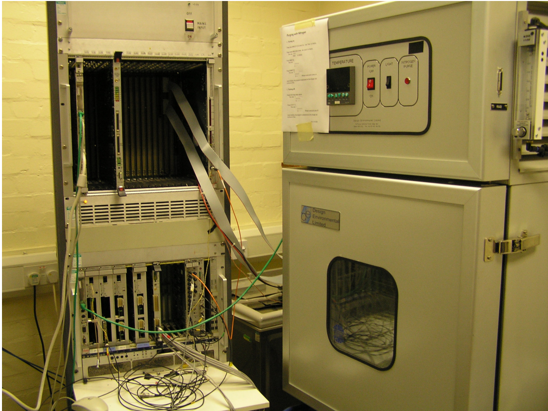
Figure 4.7: The crate and environmental chamber which housed the CPM.
