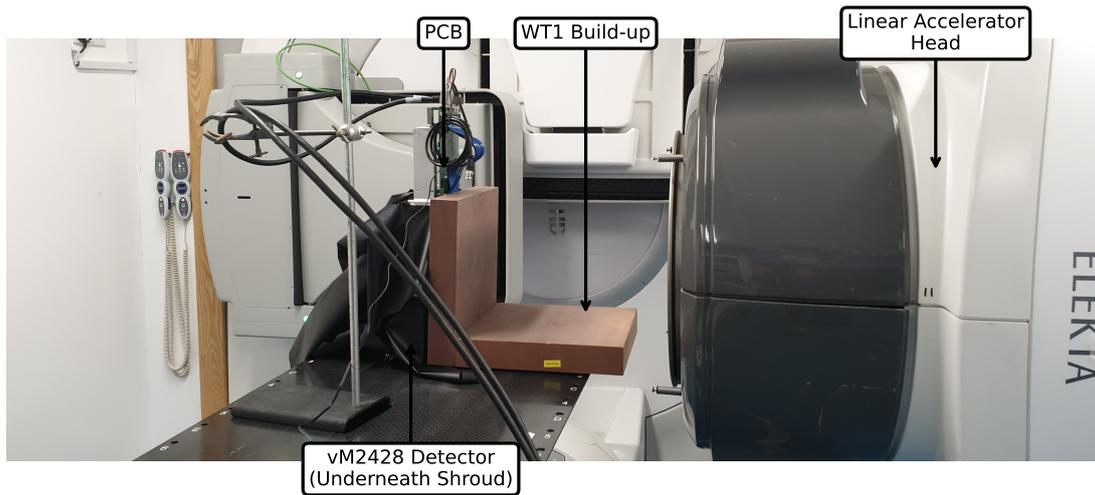
Figure 4.11: vM2428 Detector setup in Elekta Versa HD Linac for Horizontal Beam Tests.
