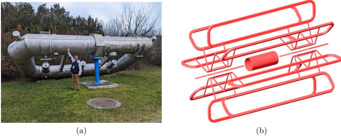
Figure 3.8: (a) Photograph of a final prototype of a toroid magnet at \simeq \frac{1}{3} scale. The prototype is displayed in front of the entrance of the ATLAS control room at CERN. A person is standing in front of the magnet for scale. (b) Schematic of the ATLAS magnet system. Both solenoid and toroidal systems are shown. Taken from Ref. [88].
