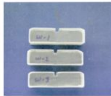
MINOS PRODUCTION BARS SHOWING 4 x 1 cm 2 CROSS SECTION WITH CO-EXTRUDED TiO 2 AND GROOVE FOR WLS FIBER
