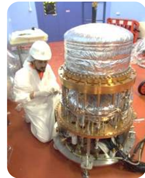
ZEPLIN: The world's first 2-phase Xenon dark matter detector (Finished 2011)
