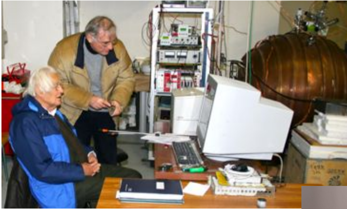
I. Giomataris and G. Charpak with a spherical proportional counter in CEA Saclay (sphere was previously a LEP RF cavity)
