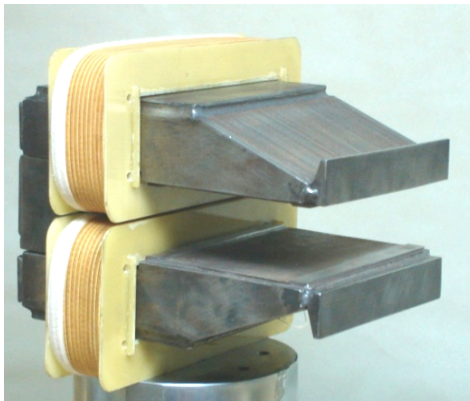
Prototypes for Ring dipoles Fabricated and tested by CERN (top) and Novosibirsk
