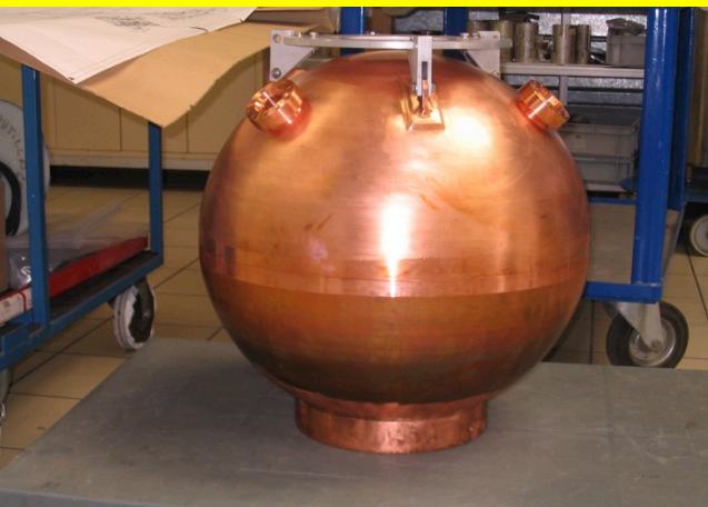
Low background detector d=60 cm p=10 bar
