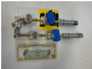
Kr-83m calibration source: Rb-83 infused into zeolite, located within xenon gas plumbing
