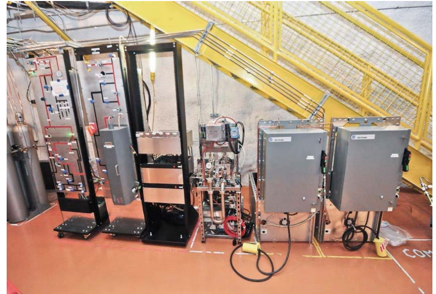
Xenon circulation system (230 kg/day)
