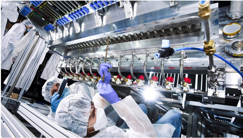
CMS Gas Electron Multiplier
